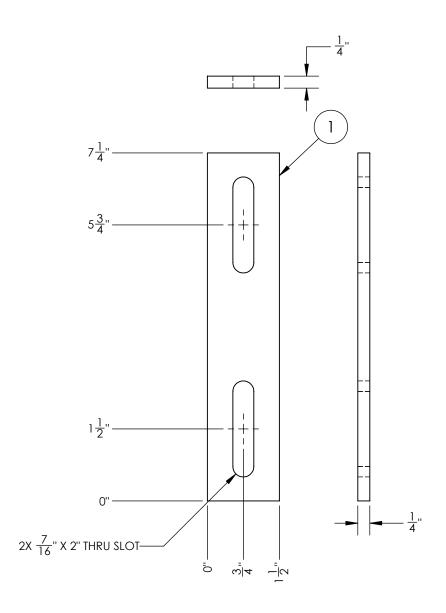
UNLESS OTHERWISE SPECIFIED: DIMENSIONS ARE IN INCHES TOLERANCE ± 1/16
