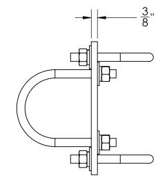
UNLESS OTHERWISE SPECIFIED: DESCRIPTION: MEDIUM CROSSOVER PLATE KIT, 2-7/8" TO 3-1/2" PIPE DIMENSIONS ARE IN INCHES TOLERANCE ± 1/16 DWG NO: PRO TOWER
